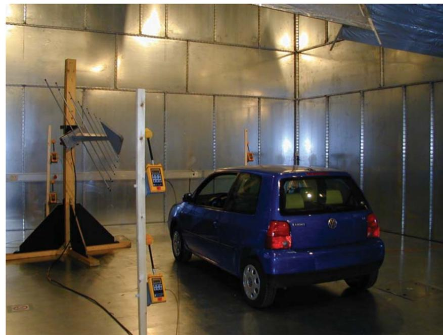
*This reverberation chamber has a test volume suitable for a regular van and can be used from about 80 MHz upwards with no upper limit. The test volume is 11.0 × 7.6 × 7.2 m<sup>3</sup>. The actual field strength is monitored by 8 field probes placed around the DUT.*
